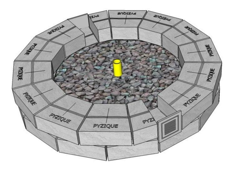
Layer 2A: Piece Count= (2) Vent Apply glue and place vents in openings on layer 2.
