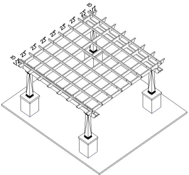
Once the rafters are installed, install the 2x4 Purlins using the 5 inch self drilling screws. Install one screw in each purlin along each of the outside rafters. Use the remaining screws to fasten the middle of the purlins to one of the middle rafters. Space the first purlin 15 and 1/2 inches in from the tip of the rafter. Position each of the remaining purlins at 23 inches from the face of the previous purlin (23 inches equals the width of one purlin plus the distance between the purlins )
