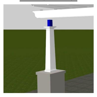
Seat Beam Assembly over Column Assembly. Place vinyl 4x4 post sleeve between the beams centered on the threaded rod. Slide the metal 4x4 post base into the post sleeve and secure to the beams with two screws on each side. Secure the post base with washer and nut over the threaded rod. **Do Not Over Tighten.**
