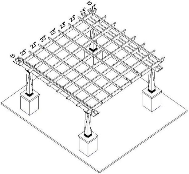
Once the rafters are installed, install the 2x4 Purlins using the 5 inch self drilling screws. Install one screw in each purlin along each of the outside rafters. Use the remaining screws to fasten the middle of the purlins to one of the middle rafters.
