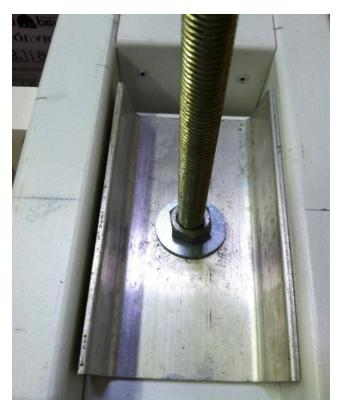
Leave bolt loosely tightened until false beam is installed. Seat Beam Assembly over Column Assembly and attach using lag screws provided.
