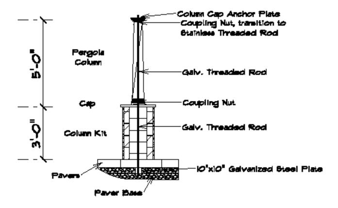
Insert threaded rod into bottom plate and attach second rod using coupling nut, then build stone column base on top of base plate.
