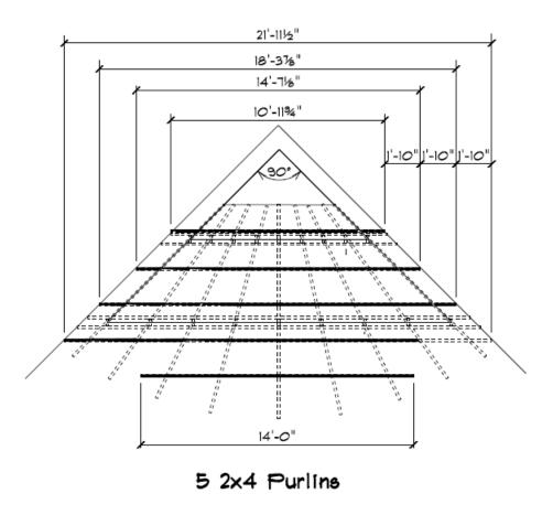
Once the rafters are installed, install the 2x4 Purlins using the 5 inch self drilling screws. Space the purlins equally using marks on the center rafter as a guide. Install one screw in each purlin along each of the outside rafters. Use the remaining screws to fasten the middle of the purlins to one of the middle rafters.
