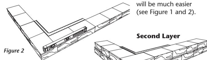
The corner will be alternated on each row with the short or long face. This will allow the bond lines of the adjoining wallstones to create extra strength. Figure 3 depicts a vertical wall application as the faces of the wallstone are positioned directly above the wallstones below them.
