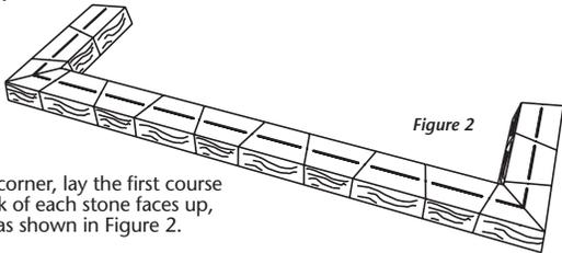
Starting with the corner, lay the first course so the center mark of each stone faces up, alternating them as shown in Figure 2.
