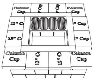
*Figure 5. Insert placement.*
