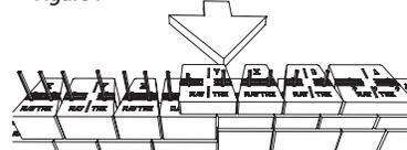
Place 6 1/2" long MaytRx Pins through the front setback hole into the center groove of the wallstone below. When the pin is centered in the hole, pull the wallstone "forward" towards the front of the wall. With the 3-inch high MaytRx wallstone, place the 3 1/4" long MaytRx Pins through the front setback hole into the center groove of the wallstone below. When the pin is centered in the hole, pull the wallstone "forward" towards the front of the wall. See Figure 7.
