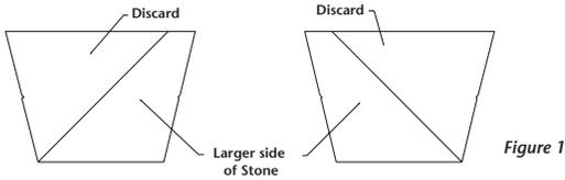
Matching 90 degree corners can be made by making a 45 degree cut in two stones starting with the corner of the smaller face on the unmarked side of the stone. The two pieces are then glued together with masonry adhesive to make a corner. These are the only cuts needed if the length equals full stones on the first layer. See Figure 1.
