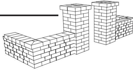
lay flat. For micro-leveling and to help the wallstones lay flat, keep a bag of sand handy and use small handfuls to level and stabilize the first layer. Start from the Olde English Radius corner detail in Figure 2 and work out from that point in each direction, alternating long and short faces. Keep the center, front and rear faces lined up to insure the wall is straight. This layout will repeat exactly for layers with odd numbers (1, 3, 5, 7, etc.) (see Figure 3).
