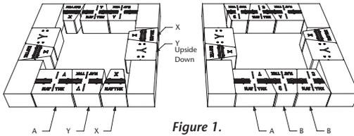
*Figure 1. Layer 1 / Wallstone placement.*
