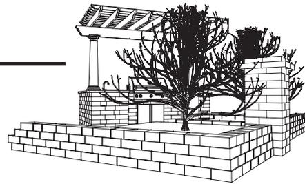
Use the visual alignment system to maintain setback from the row below 3/8". All long fronts face forward. Put the adjustment cut wallstone next to the small face of the corner. Note: Adjustment wallstones are needed to maintain the bond on the row that adjoins the small side of the corner. Lay all wallstone edges above the middle of the wallstones below except the wallstone next to the corner. Cut the adjustment wallstone to fit the space with a masonry saw.
