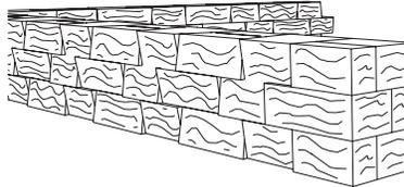
layer that will be the same as the first (Layer 1). Use a level to maintain height. Alternate front and rear faces and flip the wallstones as in all previous layers. Continue to alternate the corner and build the wall to the height desired following the odd & even formula.
