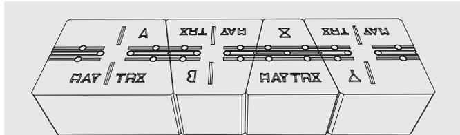
Use any combination of A, B, X or Y. The pallet contains equal amounts of each wallstone. **Note:** MaytRx wallstones can be turned upside down to fit in a random pattern, which is acceptable in the double-sided configuration.
