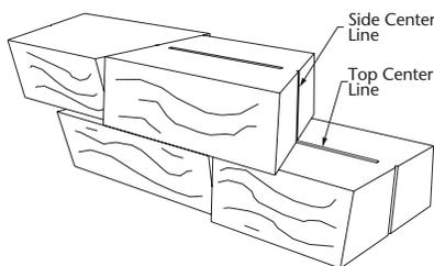
**Note:** Because the imprinted texture style of the Ledgestone Radius creates variation of the face widths on each side — much like real stone — the wallstone will align using the center top and side marks to keep the wall straight.
