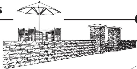
The LedgeStone Wall can also be installed setting each row back from the layer below by 3/8-inch as shown in Figure 4. This 7-degree batter creates a stronger wall in places where soil conditions or loads need a margin of safety.
