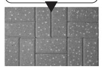
In pavers without ArmorTec, beauty is compromised when the surface reveals small stones (aggregate) after only one year of ordinary wear.
