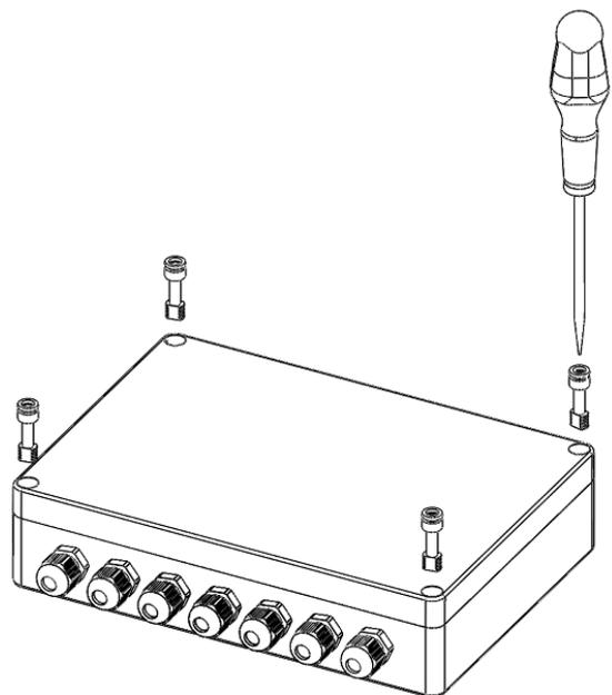
2. Use the lid as a template to mark the fixing points on the vertical wall.
