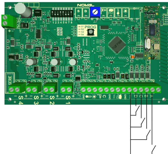
The 4 outputs S1/S2/S3/S4 can be controlled via the wired inputs A/B/C/D on the electronic board.
