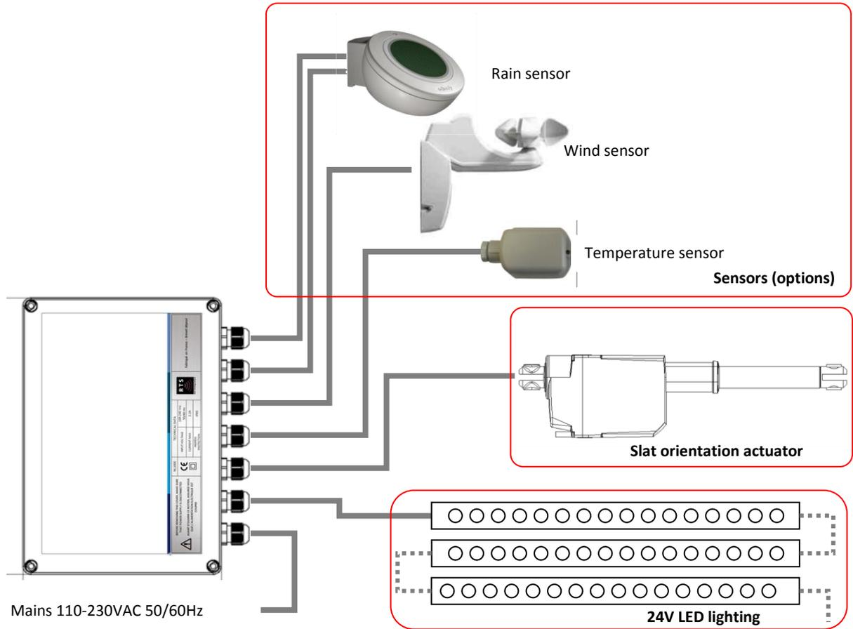
Wiring diagram for several actuators
